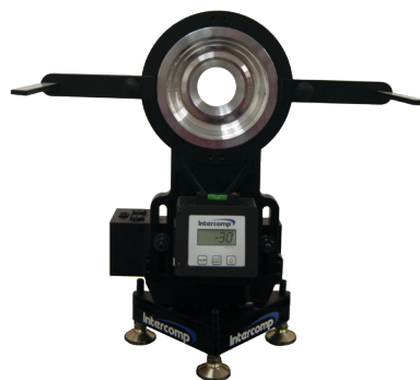
Precision CNC-machined hub stands from 6061-T6 billet aluminum with magnetic inset to incorporate Digital Caster/Camber Gauge use.
